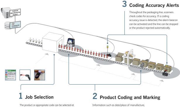
The product or appropriate code can be selected at the CLARiSUITE-installed PC or Videojet printer. Or, a bar code can be scanned from a work order or from the product itself with a hand-scanner.
